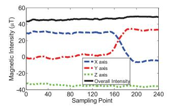
Fig. 5. Changes of magnetic intensities when the holder turns around.
