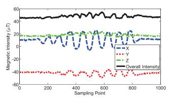
Fig. 6. Changes of magnetic intensities when the holder shakes body.
